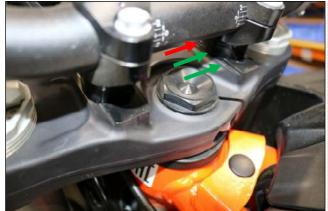
Handlebar in most forward position may cause interference at full steering lock (not recommended)
