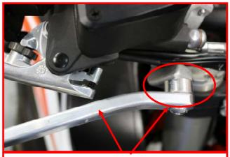
With 10mm spacer included applying the brake allows lever to operate freely.
