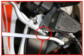
Without 10mm spacer applying the brake may cause lever to contact alloy backbone
