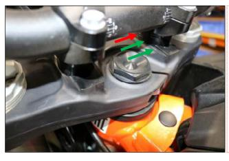
Handlebar in most forward position may cause interference at full steering lock (not recommended)
